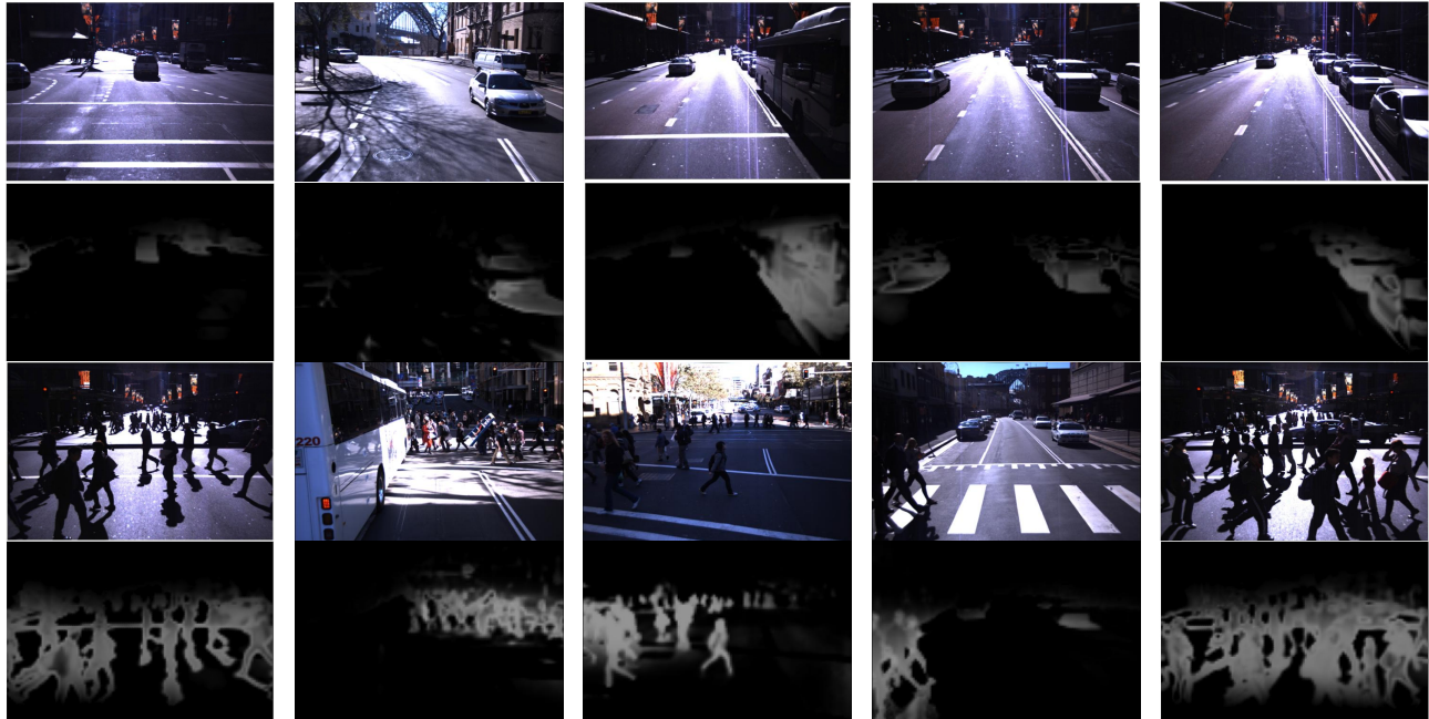
Fig. 3: Automatic dynamic object segmentation results. Each pixel has a color ranging from black (static) to white (dynamic), according to its probability of belonging to either class.
