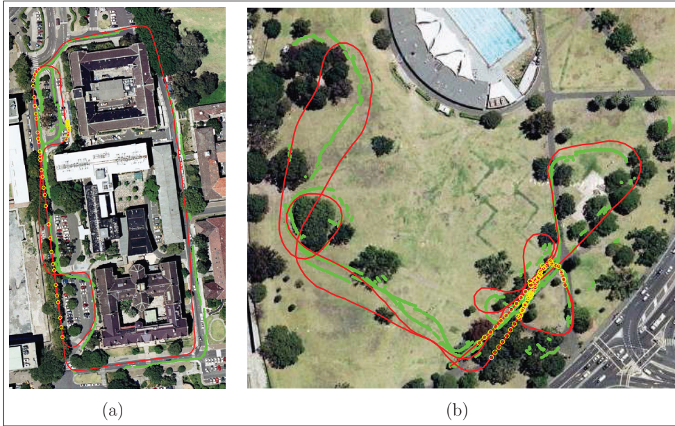
Fig. 17. Localization results obtained using the MCGP results combined with ESIF (green dots are GPS information, red lines are the localization results and yellow circles are loop-closures; color refers to the online version of this article): (a) urban dataset; (b) off-road dataset.
