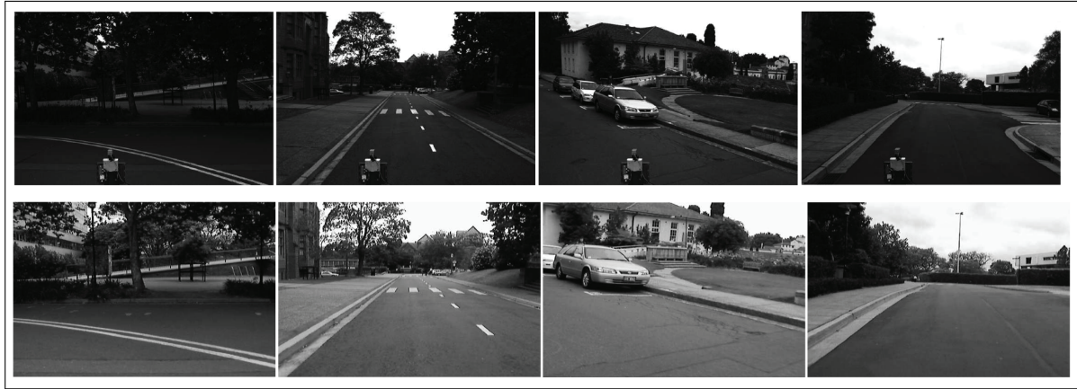
Fig. 12. Examples of images taken at the same vehicle position with different cameras. The first line corresponds to the original camera and the bottom line corresponds to the new camera (the new camera can be seen in the images captured by the original camera). The displacement between cameras is approximately 2 m horizontally and 0.5 m vertically.
